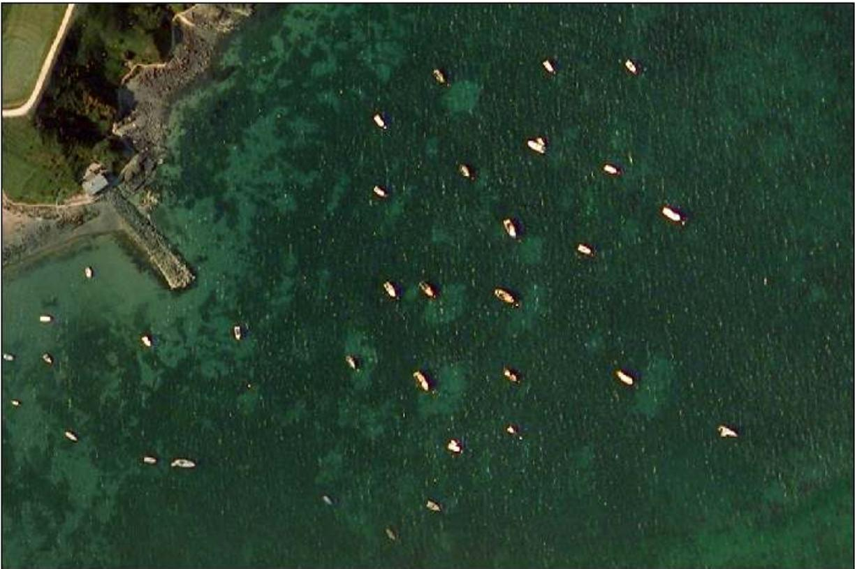
**Figure 1: Circular scars visible around traditional fixed moorings in an aerial image of Porthdinllaen. © This orthophotography has been produced by COWI A/S from digital photography captured by them in 2006. Licensed by the Welsh Assembly Government's Department for Environment.**
